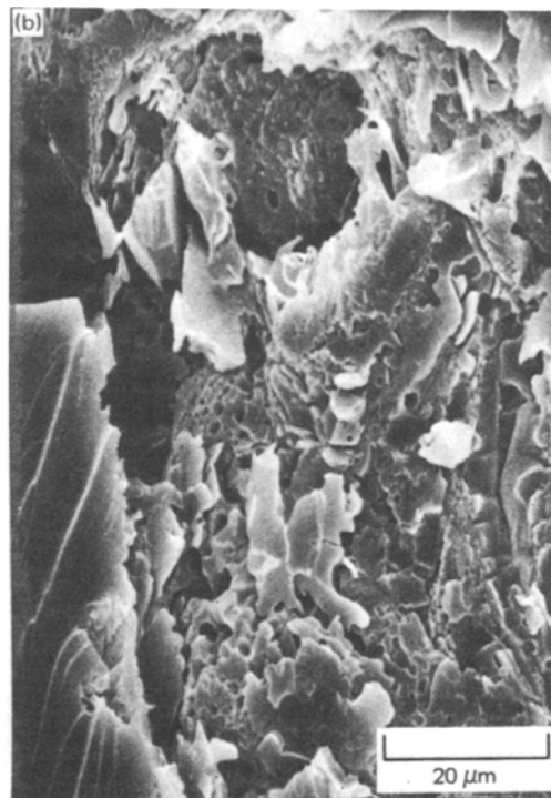
Figure 5 Scanning electron micrographs of cavities in the fracture topography initiation region of a wet TGDDM-DDS (27 wt% DDS) epoxy (~4 wt% sorbed moisture) that was fractured at room temperature at a strain rate of \sim 10^{-2} \text{ min}^{-1} .
